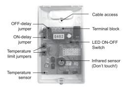
Red LED (fixed) is lit when the detector is activated. Red LED (blinking) is lit if any of the jumpers for delay is taken away.
