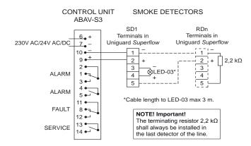
The alarm relay and the failure relay outputs are shown in alarm/no power on condition and the service alarm relay is shown in operative/no power on condition.
