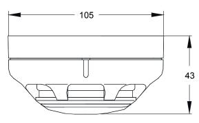
Mounting: 2 x M4 screws, 50 / 60 / 70 mm c/c
