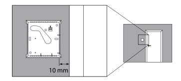
The housing has a cable entry on the backside for connection cables coming from a wall terminal box.
