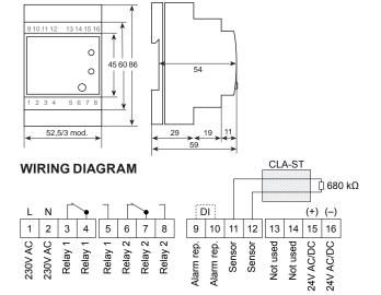
The relay outputs are shown in alarm/no power on condition. Max 5A, 250V
