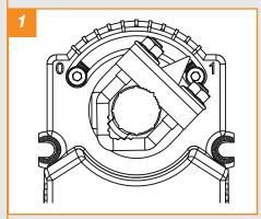
Both end stops are adjusted to 0 (0°) and 1 (90°). For smaller rotation angles, loosen the screws at the metal end stop, adjust the end stops as requested, and fasten the screws again.
