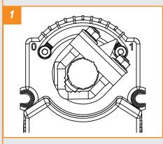
Both end stops are adjusted to 0 (0°) and 1 (90°). For smaller rotation angles, loosen the screws at the metal end stop, adjust the end stops as requested, and fasten the screws again.
