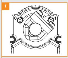
Both end stops are adjusted to 0° and 90°. For smaller rotation angles, loosen the screws at the metal end stop, adjust the end stops as requested, and fasten the screws again.
