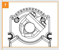
Both end stops are adjusted to 0 (0°) and 1 (90°). For smaller rotation angles, loosen the screws at the metal end stop, adjust the end stops as requested, and fasten the screws again.
